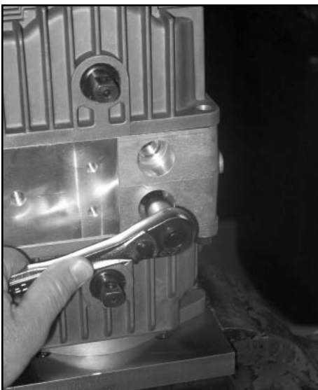
Check /shock valve removal
