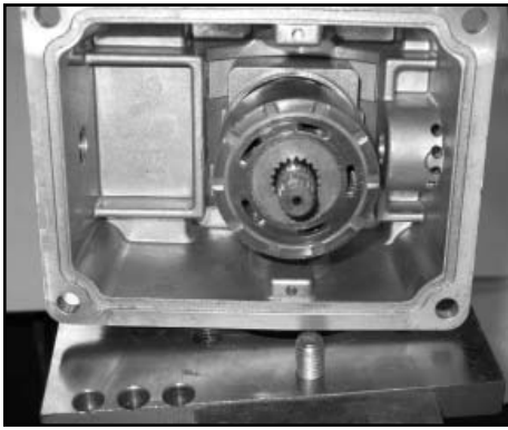
Installed rotating group
