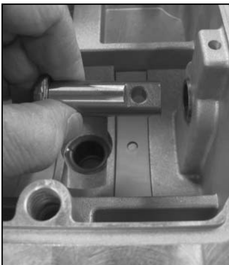
Install trunnion arms
