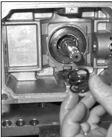
Lift off central spring
