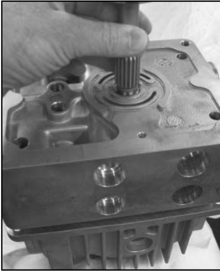
Align center block to rear housing
