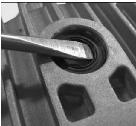
Trunnion seal removal
