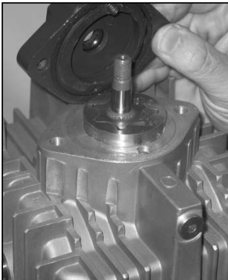
Removal of charge cover
