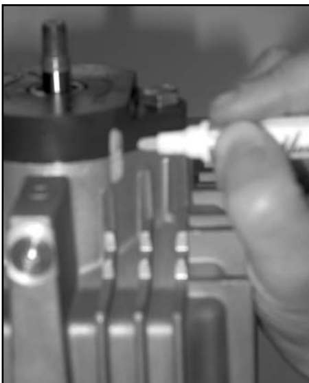
Mark charge pump cover to housing
