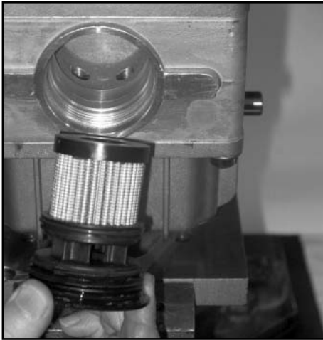
Install filter element
