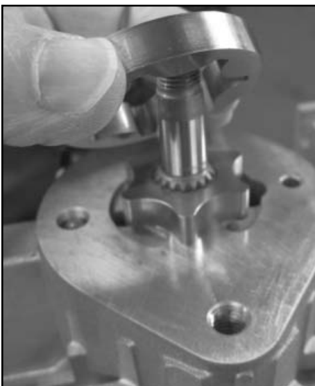
Lift off charge pump rotor set
