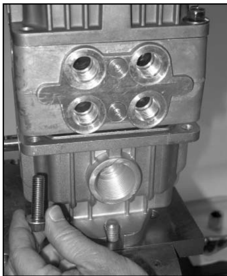
Remove front housing bolts
