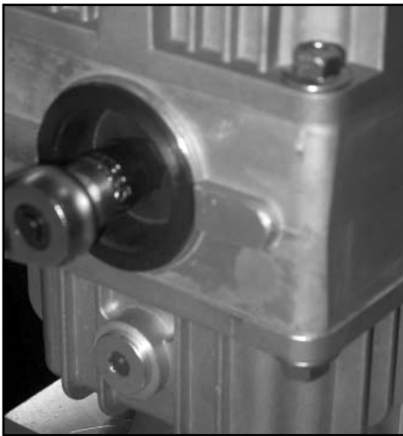
Tighten filter element
