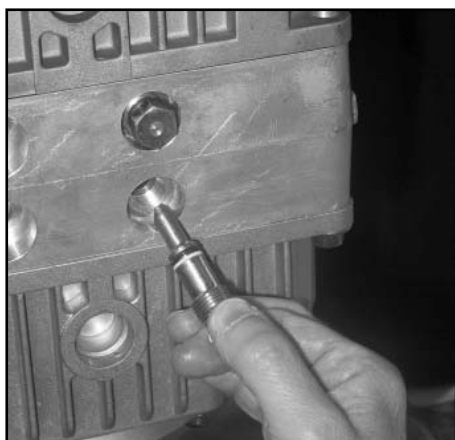
Remove bypass valves
