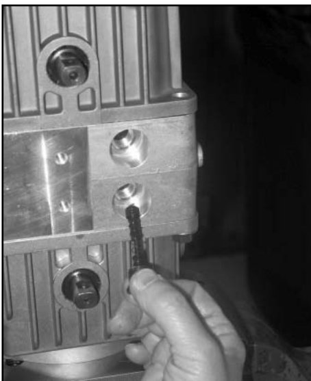
Install shock valves or check valves (depending on model)
