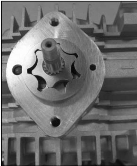
Charge rotor set installed
