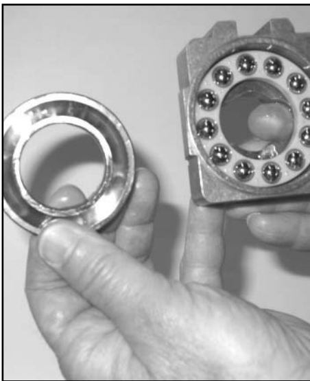
Install top bearing race
