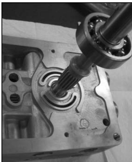
Insert shaft into front side of center block
