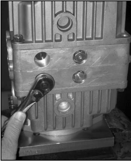
Check /shock valve removal
