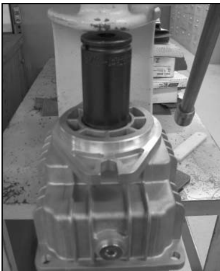
Press shaft seal into place
