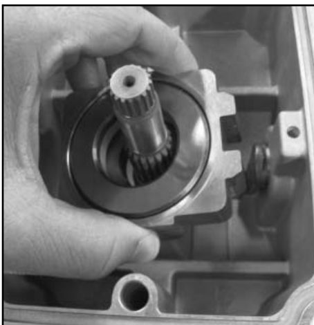
Install rear swash block
