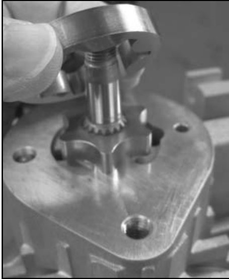
Install charge rotor set
