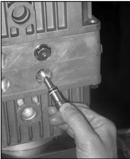
Install two bypass valves
