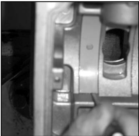
Removal of cradle bearings
