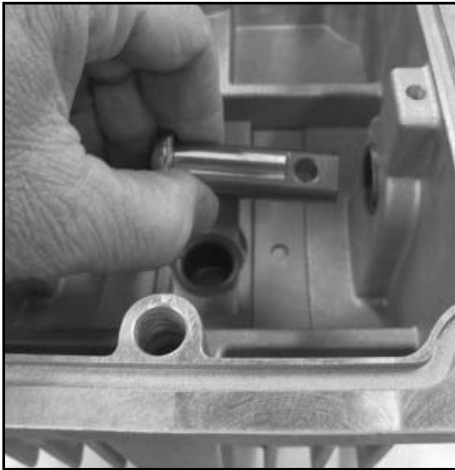
Trunnion arm removal
