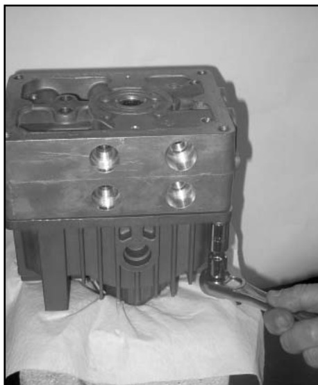
Remove bolts from rear housing and center block
