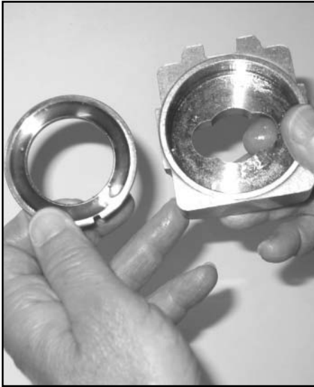
Place bottom bearing race into place
