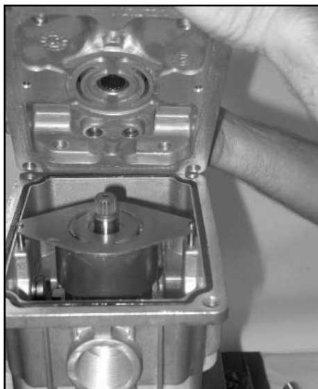
Remove center block and rear housing
