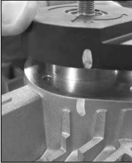
Align charge cover with marks
