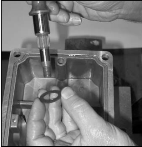
Rear shaft and washer installation
