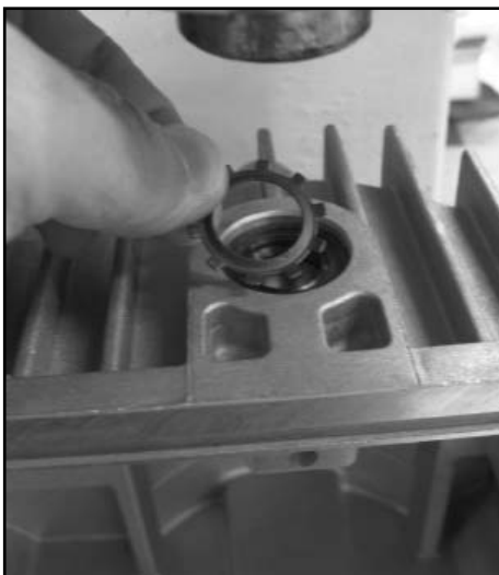
Press in seal retainers
