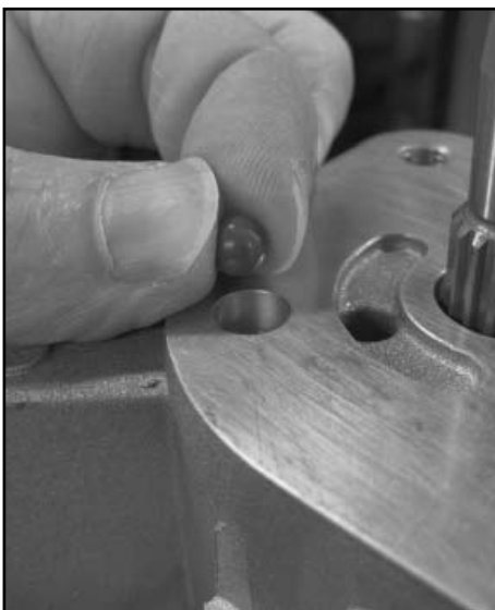
Install charge relief ball
